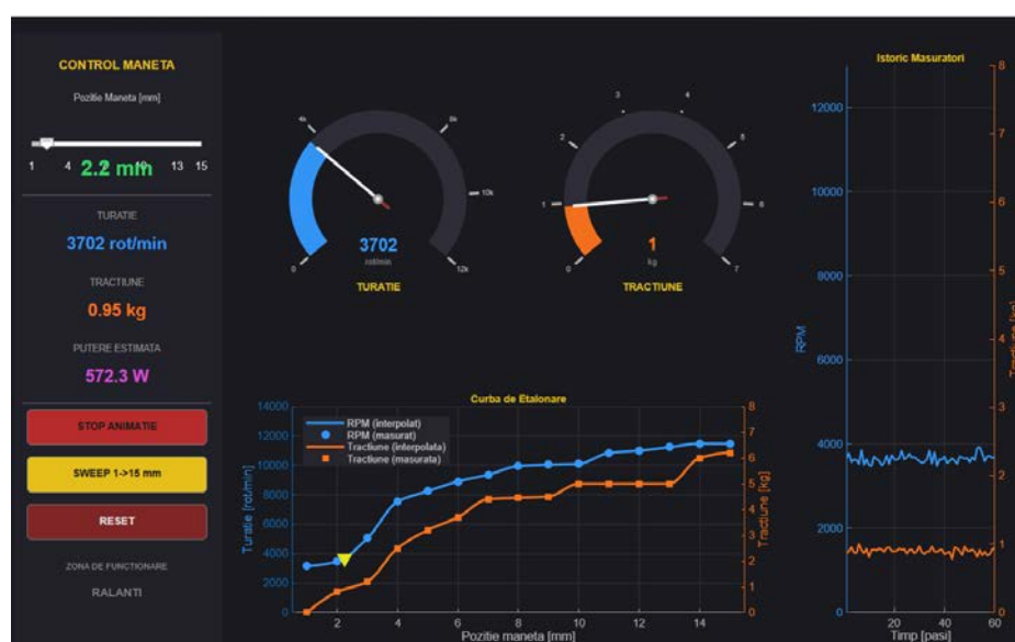
FIG.6 MatLab-Based Data Visualization and Analysis Platform
